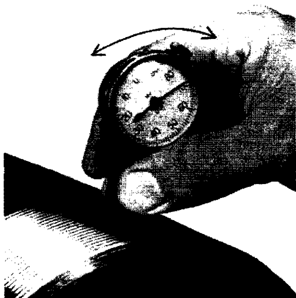
Figure 24—External/Internal Thread Height Gauge Applied to a Thread (Arcing Lines Show Direction of Rocking Motion)
