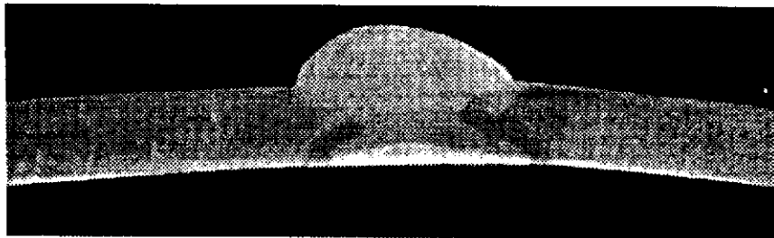
Figure 11—Excessive Reinforcement (Excessive over-fill)
