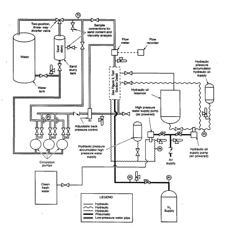
Figure 2—Example Piping Arrangement—Test Facility for PR2 Sandy Service SSV/USV Valve Verification Testing
