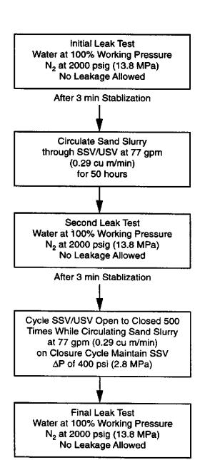
Figure 1—PR2 Sandy Service SSV/USV Verification Flow Diagram
