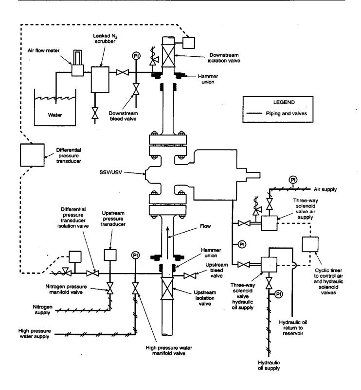
Figure 3—Example SSV/USV Valve Verification Test Section Detail
