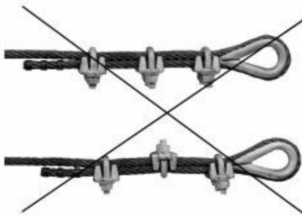
Figure 7—Incorrect Methods of Attaching Clips to Wire Rope
