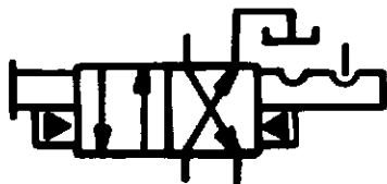
: 4 Way, Two Position, Hydraulic Pilot Operated with Manual Override, Detented Valve (fluid vent is connected to reservoir)
