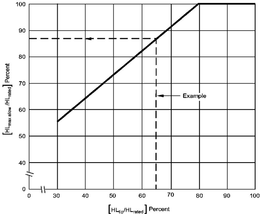
Some portable masts with guylines may have maximum rated hook load capacities ( $HL_{rated}$ ) that, if applied, could result in overloading of guyline anchors. In such cases, it is necessary to determine the maximum allowed hook load ( $HL_{max\ allow}$ ) which will prevent anchor overload. The chart above can be used to determine the magnitude of mast derating required to insure that anchor capacities shown in Figure 3 are not exceeded.
