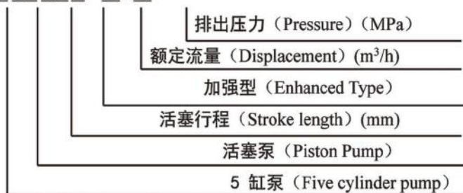
Technical specifications of 5NB series mud pump
